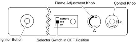
Figure 26 - Control Knob and Ignitor Button Location
